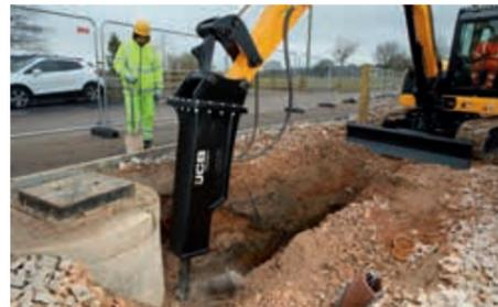
**1** To ensure correct lubrication and maximum uptime all models compatible for use on machines weighing over 11 tonnes feature a refillable auto-grease system as standard.
