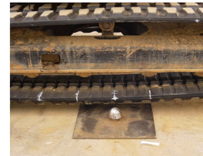
Cleat pull-out text on competitor products
