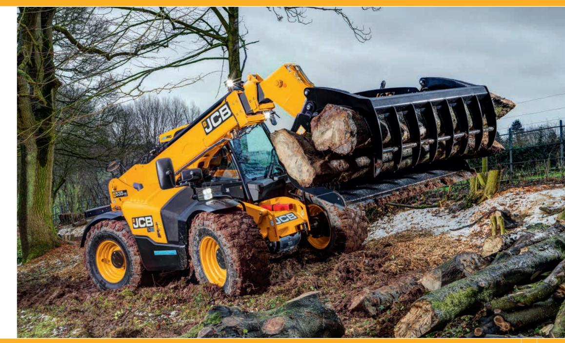
MADE OF DOMEX STEEL AND FULLY GALVANISED, THE NEW JCB BUCKET BRUSH IS DESIGNED FOR OUR RANGE OF GRAIN SHOVELS FROM 2.13M TO 2.44M. STRONGER, LIGHTER AND MORE DURABLE THAN EVER, IT STANDS UPRIGHT WHEN IT'S NOT IN USE AND ALSO HAS A QUICK-RELEASE BRISTLE CARTRIDGE.
