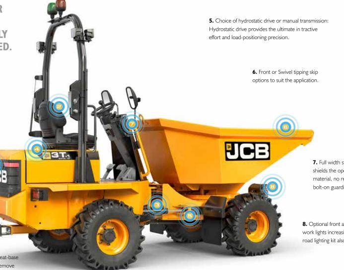
7. Full width steer column shields the operator from falling material, no requirement for bolt-on guarding.
