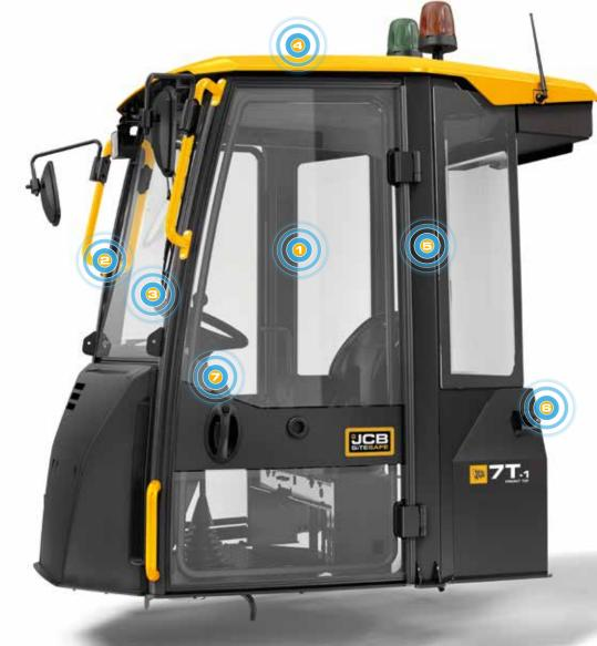
**4.** Detachable for service access and transport. When fitted to a 6 or 7 tonne dumper, overall height remains under 3m.
