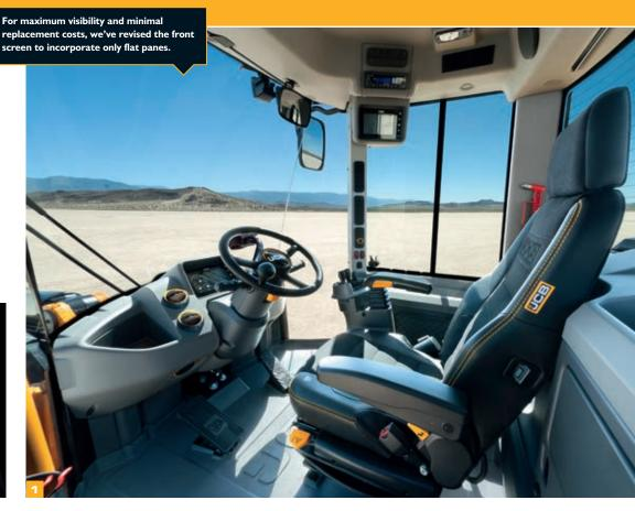
To keep the operator environment comfortable for working at all times, we've positively pressurised the cab to eliminate dust and fumes.
