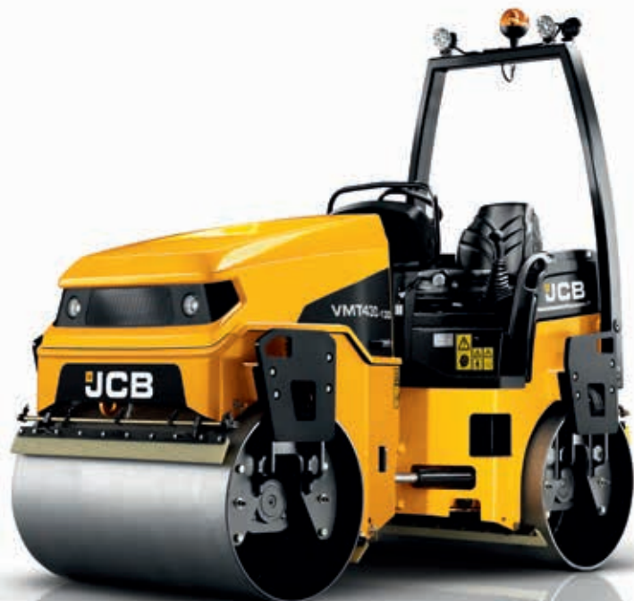
A stiff front bonnet recessed and protected by a steel bull bar gives maximum impact protection.
