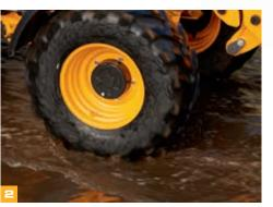
Our unique oscillating centre pivot point makes the most of traction by maintaining even weight distribution over each of the four wheels. It also gives extra stability and ride comfort.
