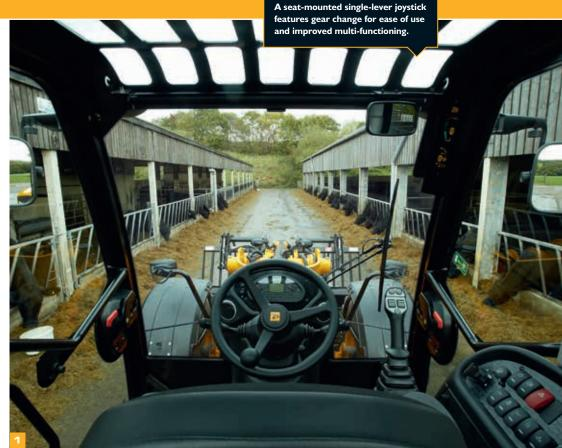
A fully adjustable telescopic steering column allows you to fine tune the driving position.
